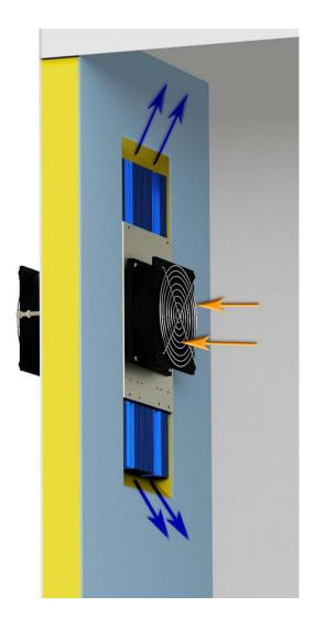
**Note**: in a condensing environment, be sure to mount the cold side heat sink fins in a vertical position in order to drain the condensation.
