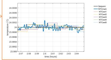
The left figure shows the measured temperatures. The black line indicates the set point temperature, and 'NTCmain' is the controlled chilled water temperature. NTCext1 to NTCext5 indicate 5 external temperatures sensors that are located in the outlet water flow of the chiller. The figure above shows that the temperature of these external sensors is kept within  $\pm 0.0005^{\circ}$ C temperature stability.
