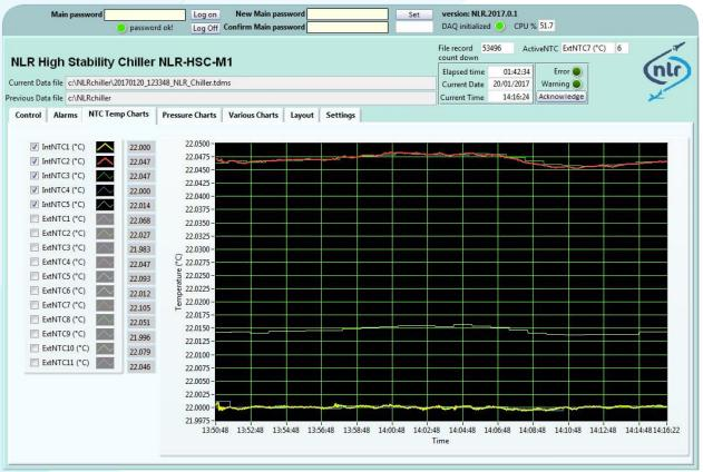
The Graphical Users Interface (GUI) can be opened in a browser on any PC that is connected to the same network as the chiller. The GUI contains displays for all the measured values (temperatures, pressures, volume flow) and is used to control the system. The measured data is automatically stored.
